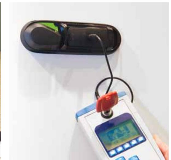
Programming unit – transfers authorizations, reads logs or opens doors if batteries run out.
